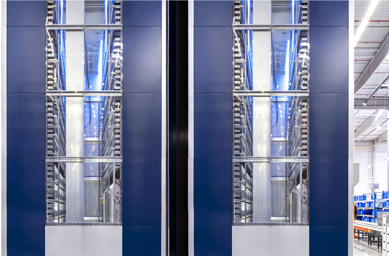
16. Plexi glass on short side, 17. Led bars inside the shaft
